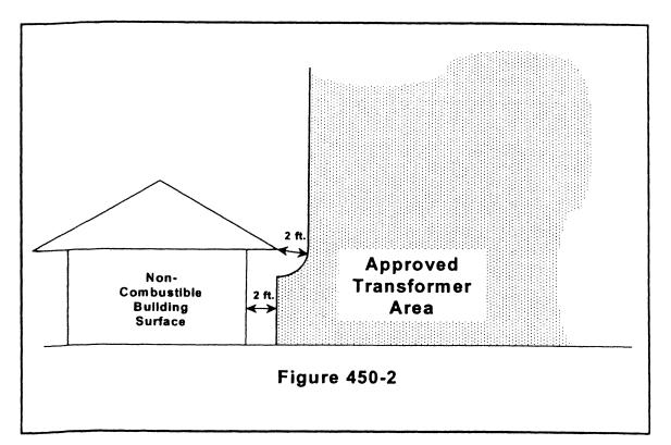
(c) In an area in which a transformer is to be installed next to a nonhabitable structure, the transformer may be no closer than two feet to the building/structure and must be outside a line extended vertically from the ends of the eaves or rooflines;
