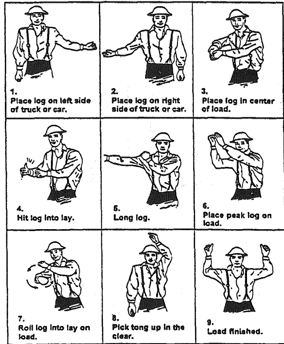
Figure 42: Standard Signals for Loading Logs
