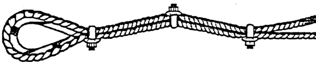
3. WRONG METHOD—Staggered clips; two correct and one wrong. (This will cause a mashed spot in live end of rope due to wrong position of center clip) 4. After rope is in service, and is under tension, tighten clips to take up decrease in rope diameter.
