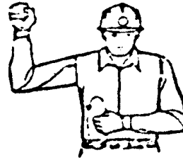
FOR MOBILE CRANES LOCK THE CRAWLER BELT ON SIDE
