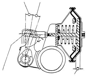
POINT OF GREATEST LEVERAGE MOVEMENT PAST THIS POINT RESULTS IN LESS LEVERAGE, REDUCED INPUT AND LOWER BRAKE EFFICIENCY. \*FIRST HALF OF RATED TRAVEL\* BRAKE CHAMBER IS AT THE MAXIMUM EFFICIENCY.
