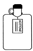
This is an example of a labeled container. You may use a laminated or coated label, affixed to the container with a wire, to avoid deterioration of labels due to a solvent, such as acetone.
