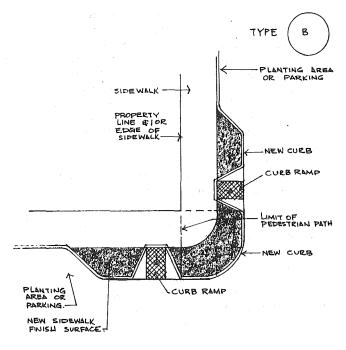
(1) This curb ramp type can be used with the existing planting area or with the sidewalk extension into the parking area.
