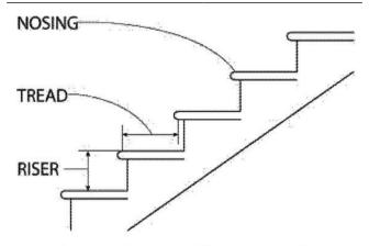
MINIMUM TREAD WIDTH 22 IN (56 CM) MINIMUM TREAD DEPTH 9.5 IN (24 CM) MAXIMUM RISER HEIGHT 9.5 IN (24 CM)
