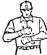
FOR MOBILE CRANES HOIST THE LOAD AND LOWER THE BOOM
