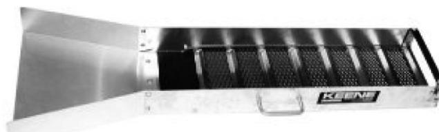
**Figure 8: Sluice**
