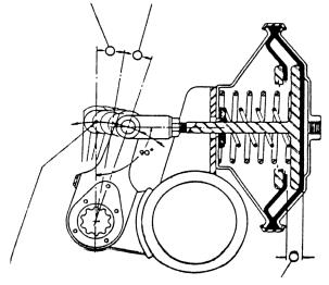
POINT OF GREATEST LEVERAGE MOVEMENT PAST THIS POINT RESULTS IN LESS LEVERAGE, REDUCED INPUT AND LOWER BRAKE EFFICIENCY.
