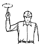
HOIST THE LOAD
