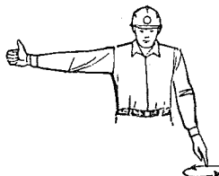
FOR MOBILE CRANES LOWER THE LOAD AND RAISE THE BOOM
