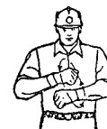
FOR MOBILE CRANES TRAVEL BOTH CRAWLER BELTS IN DIRECTION INDICATED BY REVOLVING FISTS
