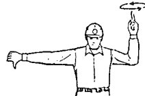
SWING LOAD IN DIRECTION FINGER POINTS
