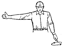
FOR MOBILE CRANES LOWER THE LOAD AND RAISE THE BOOM
