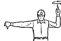
SWING LOAD IN DIRECTION FINGER POINTS
