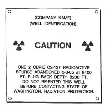
The size of the plaque should be convenient for use on active or inactive wells, and shall be at least eighteen centimeters square. Letter size of the word "CAUTION" or "DANGER" shall be approximately twice the letter size of the rest of the information, e.g., one-half inch and one-fourth inch letter size, respectively.
