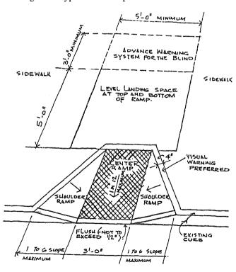
Texturing of center ramp recommended, with metal grid placed in wet concrete and then removed to leave ridged surface pattern. Pattern not to exceed 1/2" width. (2) Advance warning strip (shown dotted), necessary when ramp is in direct line of main pedestrian path.
