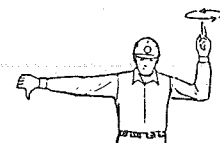
FOR MOBILE CRANES HOIST THE LOAD AND LOWER THE BOOM
