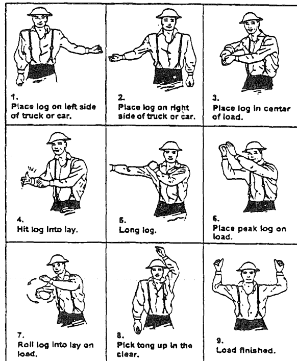
Figure 42: Standard Signals for Loading Logs
