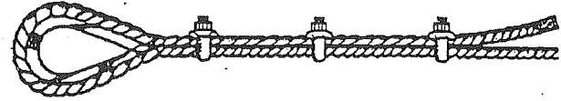
2. WRONG METHOD – U-Bolts on live end of rope. (This will cause mashed spots on live end of rope)
