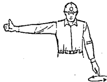
FOR MOBILE CRANES LOWER THE LOAD AND RAISE THE BOOM
