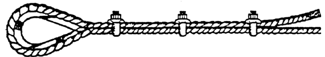
2. WRONG METHOD—U-Bolts on live end of rope. (This will cause mashed spots on the live end of rope)
