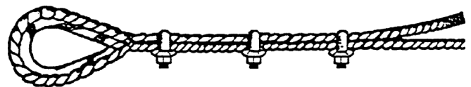
1. CORRECT METHOD—U-Bolts of clips on short end of rope. (No distortion on live end of rope)
