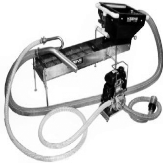
Figure 5: Power sluice/suction dredge combination
