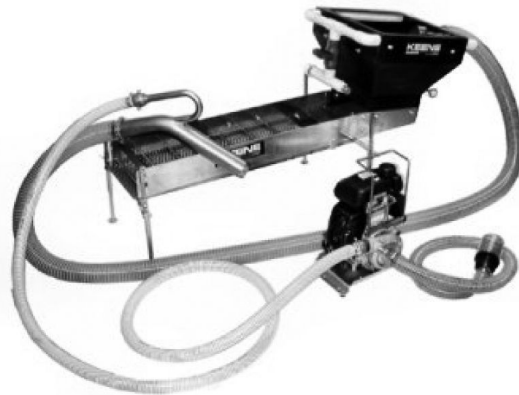
Figure 5: Power sluices/suction dredge combination
