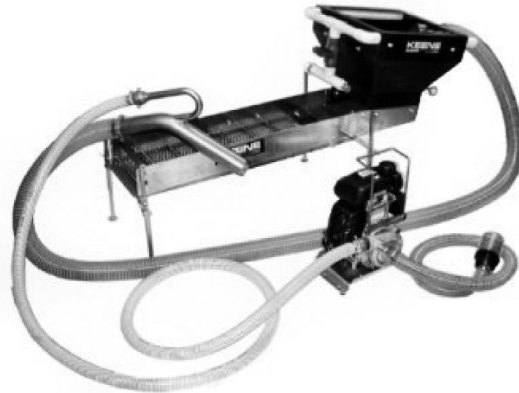
Figure 5: Power sluices/suction dredge combination
