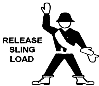
Left arm held down away from body. Right arm cuts across left arm in a slashing movement from above.
