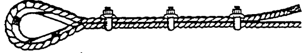
2. WRONG METHOD – U-Bolts on live end of rope. (This will cause mashed spots on live end of rope)
