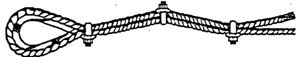
3. WRONG METHOD – Staggered clips; two correct and one wrong. (This will cause a mashed spot in live end of rope due to wrong position of center clip)
