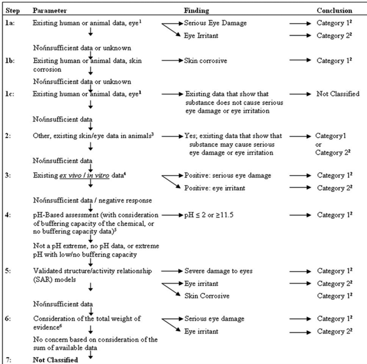
Figure A.3.1 Evaluation strategy for serious eye damage and eye irritation (See also Figure A.2.1)
