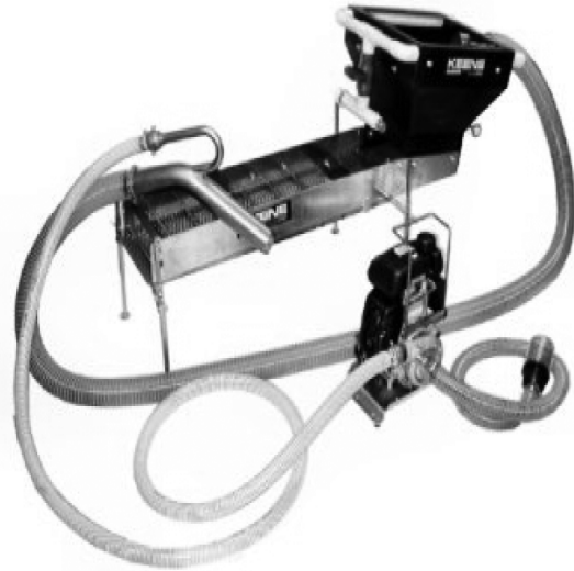
Figure 5: Power sluices/suction dredge combination
