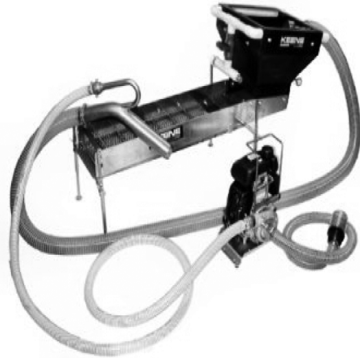
Figure 5: Power sluice/suction dredge combination
