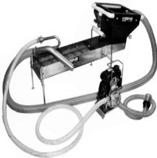
Figure 5: Power sluices/suction dredge combination
