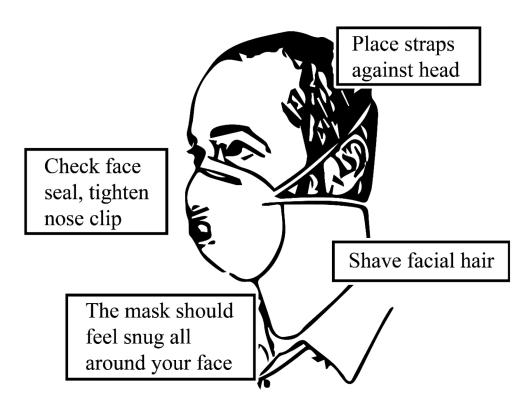
For a respirator that relies on a tight seal to the face, check how well it seals to the face by following the manufacturer's instructions for user seal checks. Adjust the respirator if air leaks between the seal and the face. The more air leaks under the seal, the less protection the user receives.
